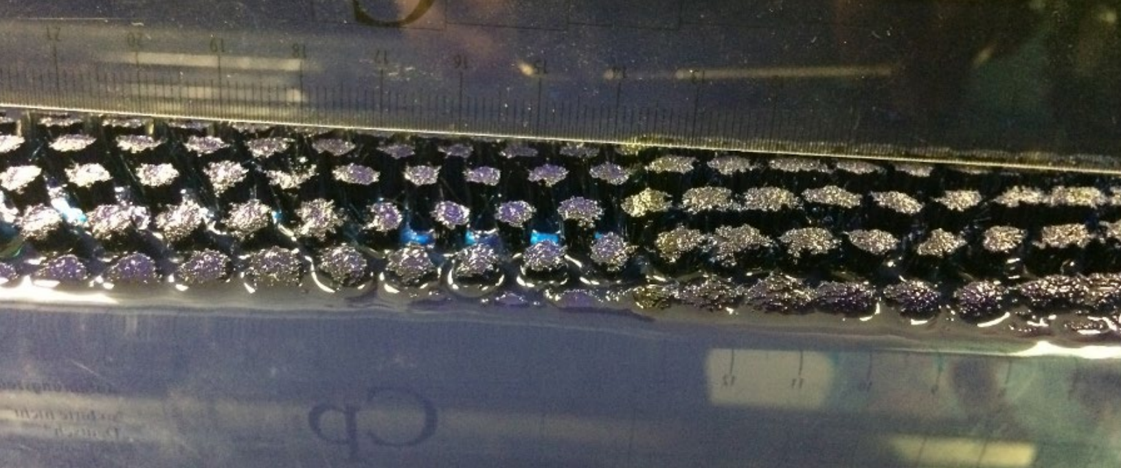
Figure 5: Worn out developer brush
