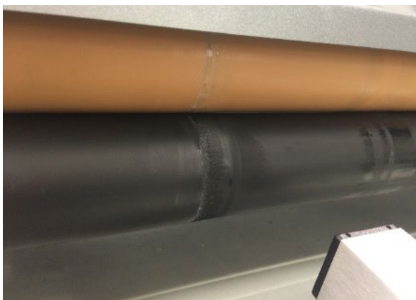
Figure 7: Dry residues on the roller's surface
