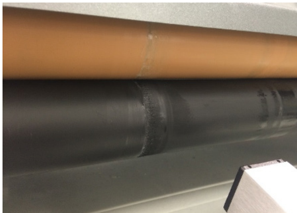
Figure 7: Dry residues on the roller's surface
