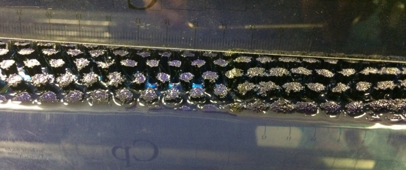
Figure 5: Worn out developer brush
