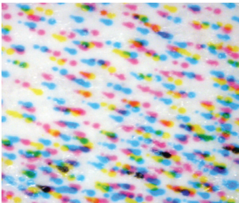
Figure 3: Kodak Stream drop placement: Comparison between Kodak drops (Left) with DOD (Right).
